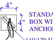
STANDARD 4" ROUND OR SQUARE PANCAKE BOX WITH HANGAR BAR. USE PROPER ANCHOR BOLTS/LAG BOLTS TO SECURE.
