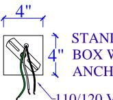
STANDARD 4" ROUND OR SQUARE PANCAKE BOX WITH HANGAR BAR. USE PROPER ANCHOR BOLTS/LAG BOLTS TO SECURE.
